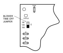
The control is factory set to give a (150) second blower off delay. See drawing below for the jumper position for all available settings:
